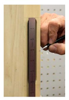
Measure the distance between the top and bottom of the mortise and divide by two.
