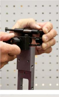
Loosen the black plastic knob until you can rotate the vise block 180 degrees, this will allow it to rotate freely. Repeat this procedure with the other end of the clamp.
