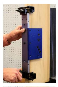
To attach the clamp, just slide over the post and tighten to the door.
