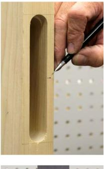
Make a mark at this point, this will be the center of the mortise pocket and the center of the mortise faceplate.
