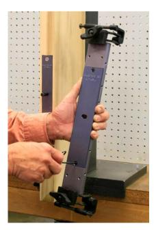
One half of the template will screw to the face of the HIT-45 clamp as shown. Be sure to use the shorter (1/2" long) of the screws supplied.
