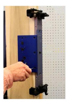
This clamp can be used with one or two templates. If using only one template prep one side of the door and with the clamp still in position, remove the template and install on the other side.
