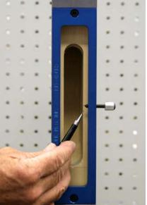
Hold the HIT-45 to the door with the locating pointer pointing to the center line, allow the bevel blocks to conform the door bevel and tighten clamps. Double check the pointer is located to center and remove the pointer.
