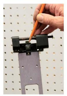
There is a backset stud located in the center of the top and bottom clamp. It will set the correct backset calculated from the center of the door regardless of door bevel.
