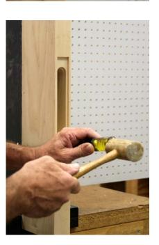
Use a standard chisel to finish removing the round corners and final cleanup.
