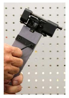
Attach the bevel blocks both top and bottom on the inside of the HIT-45 clamp with the supplied 10-32 x 1/2" flat head socket screws. These blocks pick up the door bevel.
