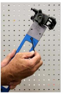
Install the HIT-45AR5 template using the supplied 10-32 x 1/2" long flat head socket screws. Using a 5/8" router template guide and a 1/2" router bit, this template will route a 1-1/4" wide x 8" tall faceplate.
