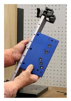
When attaching the mortise lock template to the clamp, be sure the center hole of the template is fastened to the center hole of the clamp.
