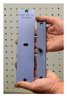
Shown is the HIT-45ML1 alignment fixture. This is used to align the function holes used by the mortise lock to the correct location in the mortise pocket. It will work with any of our mortise lock templates that use a 1-1/4" wide by a 8" tall faceplate.
